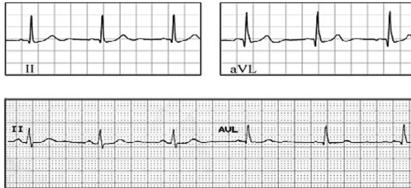
Fig. 4 Comparison of two vectors from a pair of EPIC sensors (top) and two conventional Ag/AgCl electrodes (bottom)
