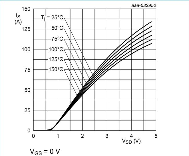
Fig. 18. Source-drain (diode forward) current as a function of source-drain (diode forward) voltage; typical values
