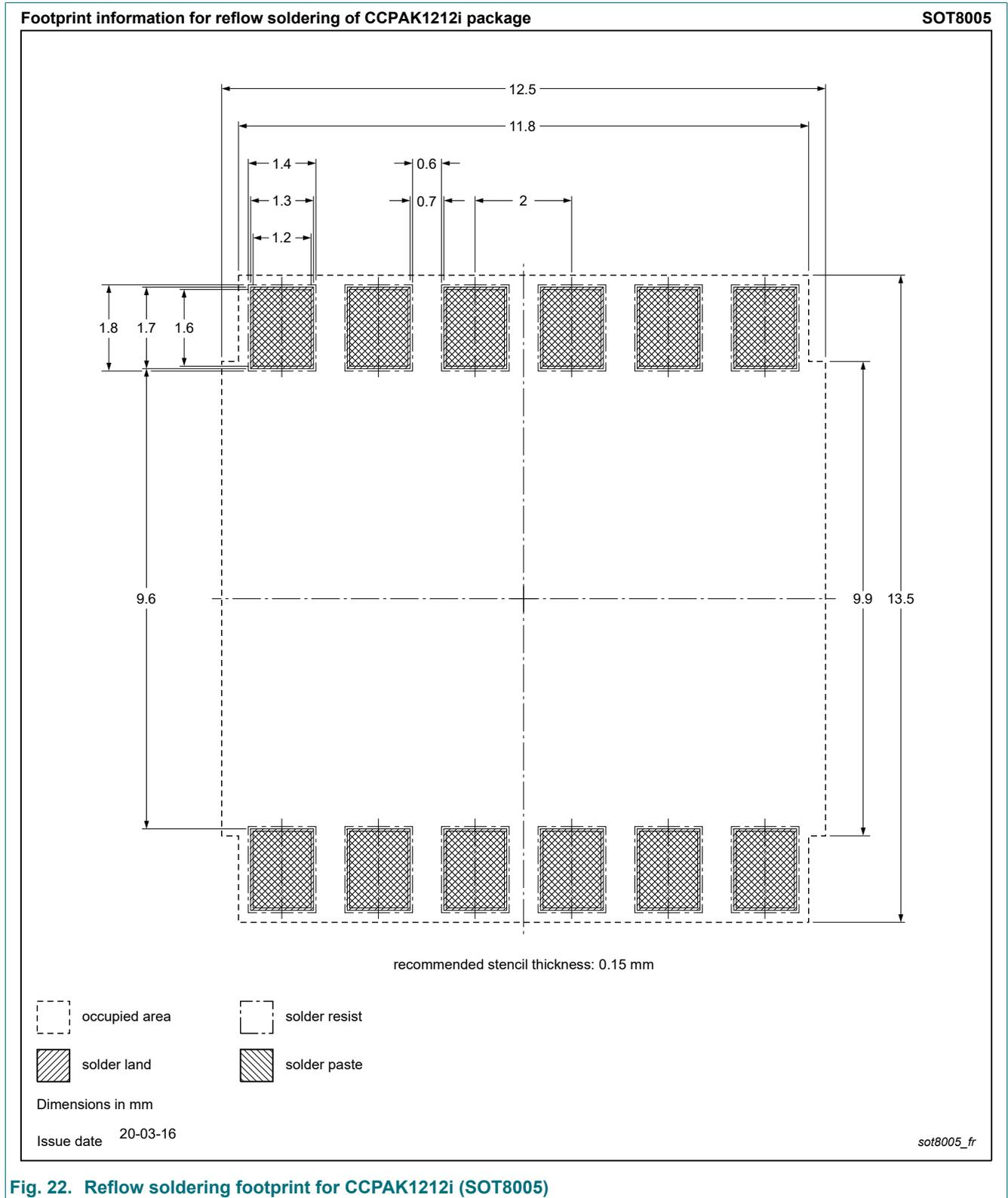
Fig. 22. Reflow soldering footprint for CCPAK1212i (SOT8005)
