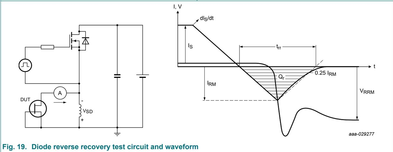
Fig. 19. Diode reverse recovery test circuit and waveform
