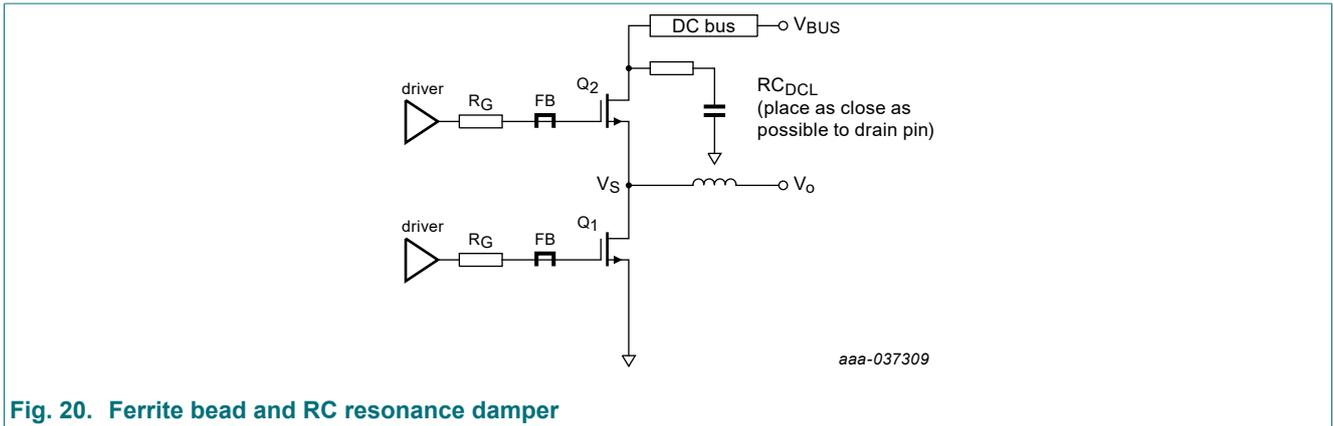
**Fig. 20. Ferrite bead and RC resonance damper**
