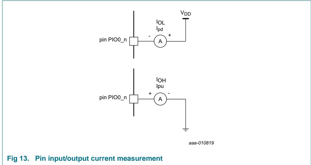
Fig 13. Pin input/output current measurement
