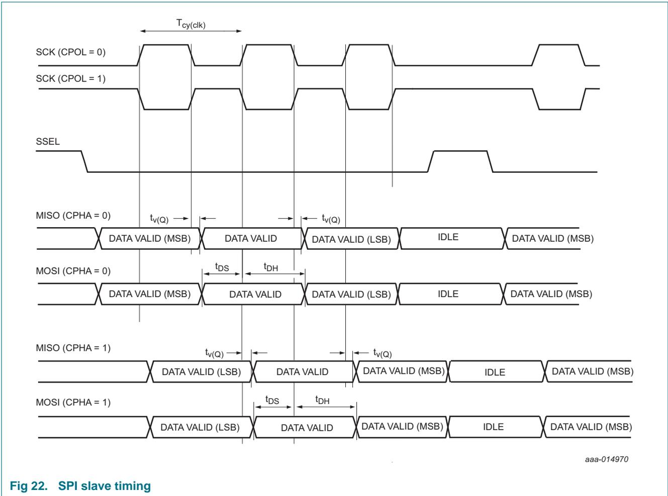
Fig 22. SPI slave timing
