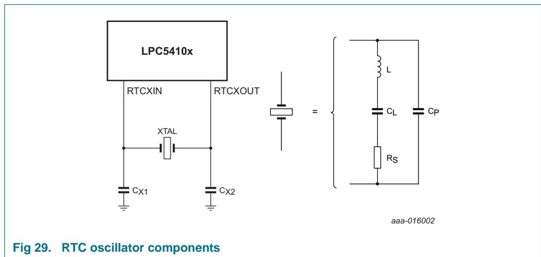
Fig 29. RTC oscillator components
