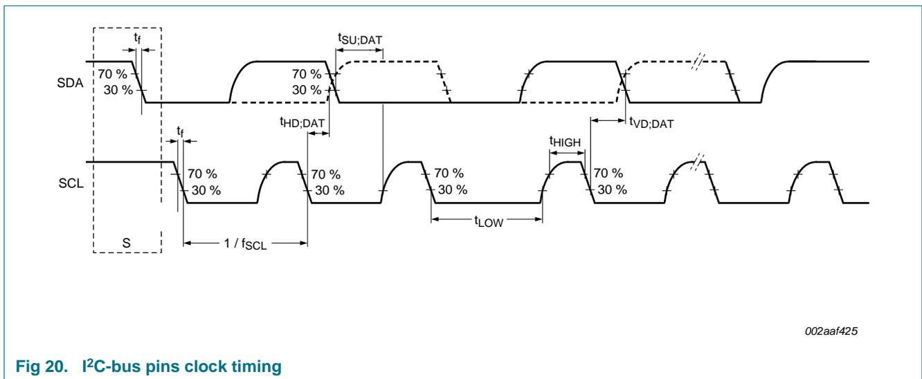
Fig 20. I<sup>2</sup>C-bus pins clock timing
