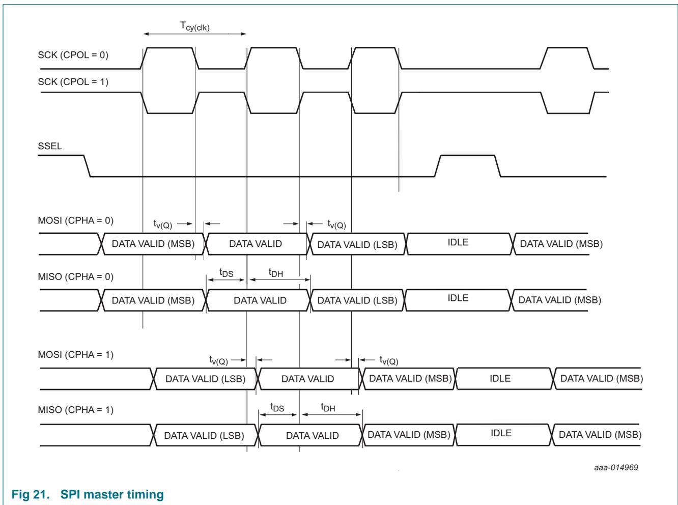
**Fig 21. SPI master timing**
