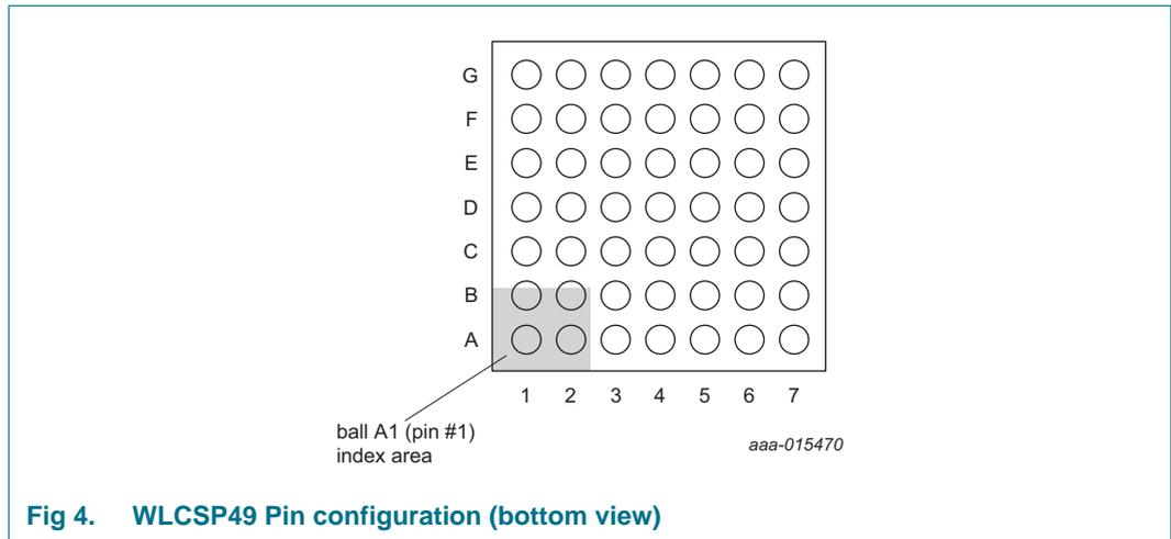
Fig 4. WLCSP49 Pin configuration (bottom view)
