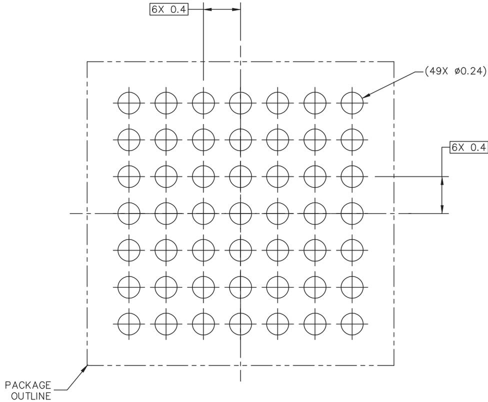
PCB DESIGN GUIDELINES – I/O PADS AND SOLDERABLE AREA
