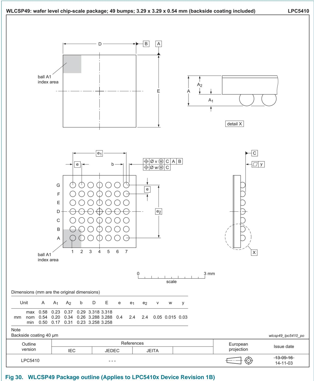
Fig 30. WLCSP49 Package outline (Applies to LPC5410x Device Revision 1B)
