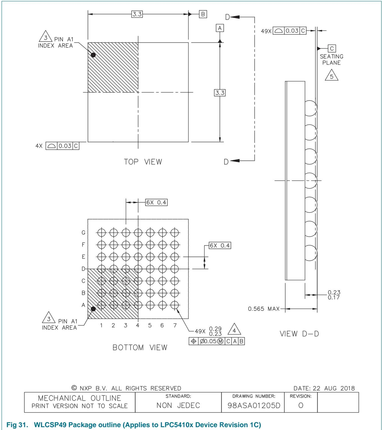
Fig 31. WLCSP49 Package outline (Applies to LPC5410x Device Revision 1C)
