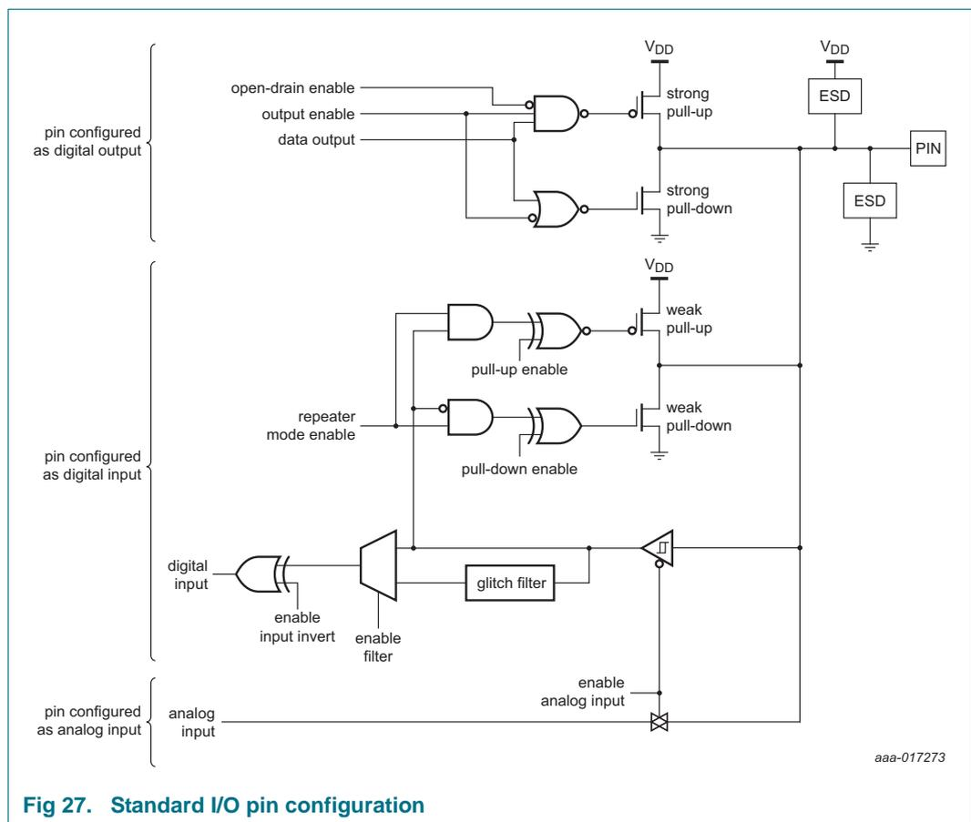
Fig 27. Standard I/O pin configuration
