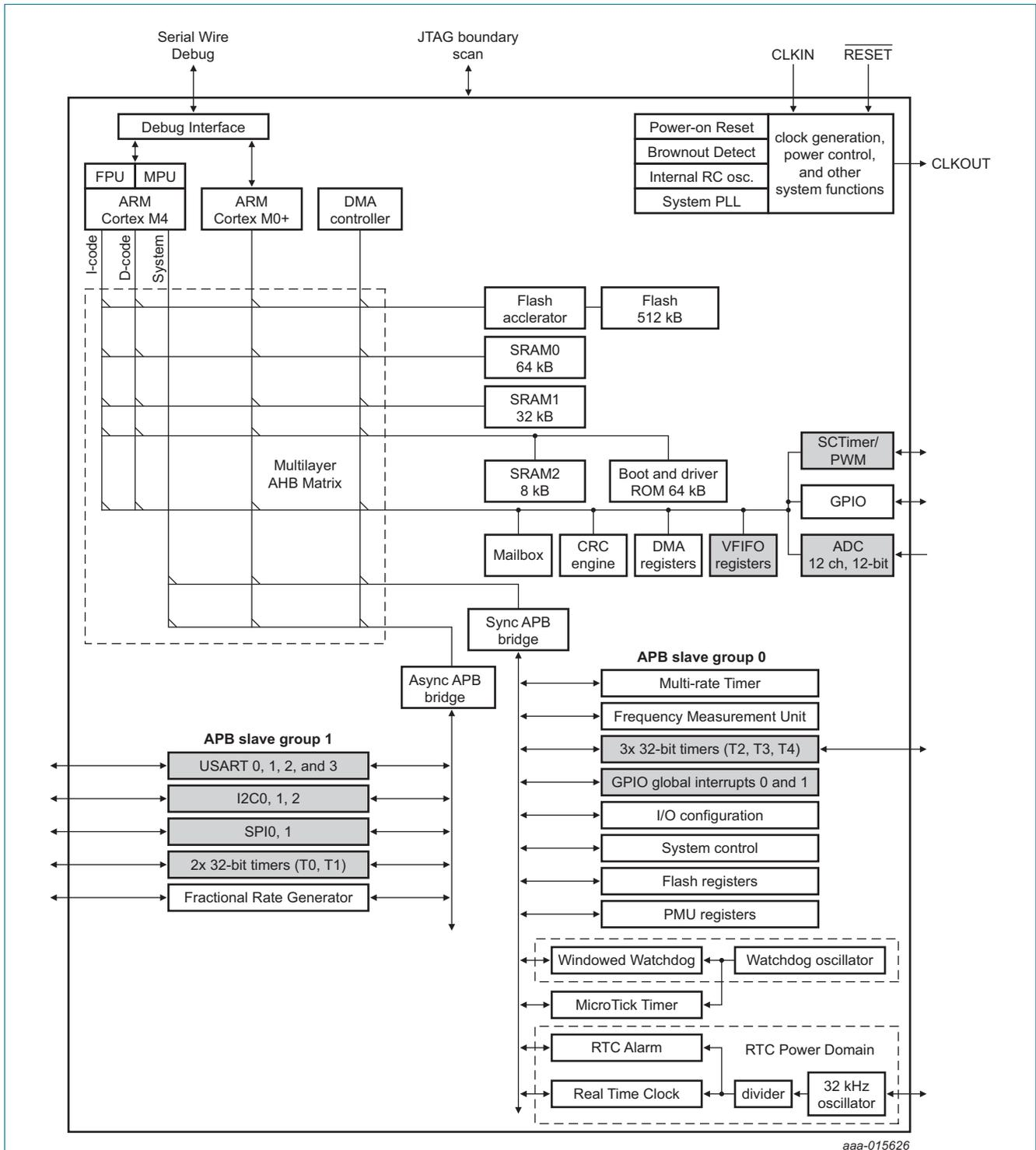
Gray-shaded peripheral blocks provide dedicated request lines or triggers for DMA transfers.
