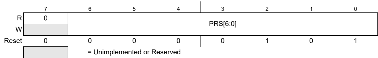
Figure 9-7. ADC Timing Register (ADCTIM))
