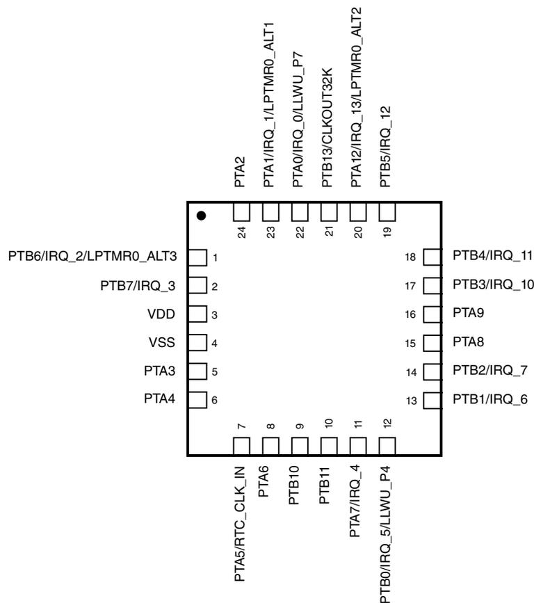
Figure 18. MCX C041 24-pin QFN pinout diagram
