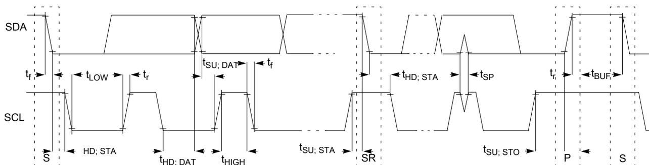
Figure 17. Timing definition for devices on the I<sup>2</sup>C bus
