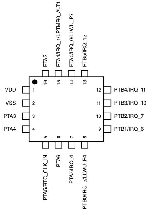
Figure 19. MCX C041 16-pin QFN pinout diagram
