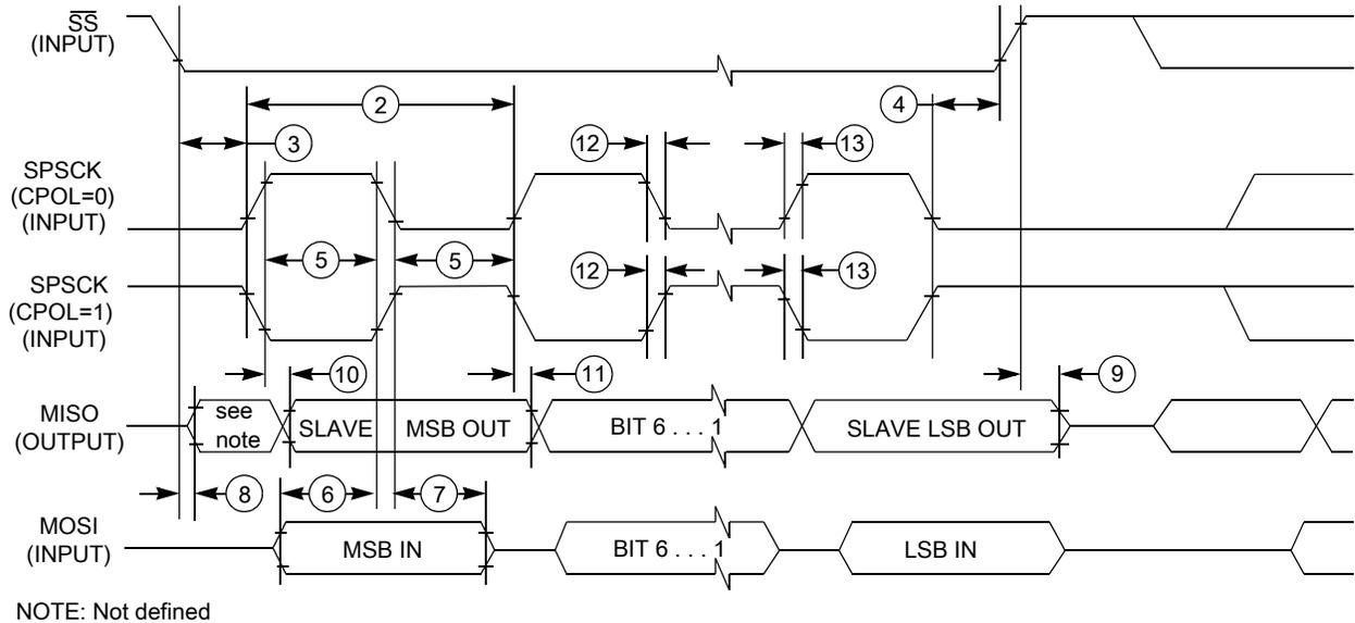
Figure 16. SPI slave mode timing (CPHA = 1)
