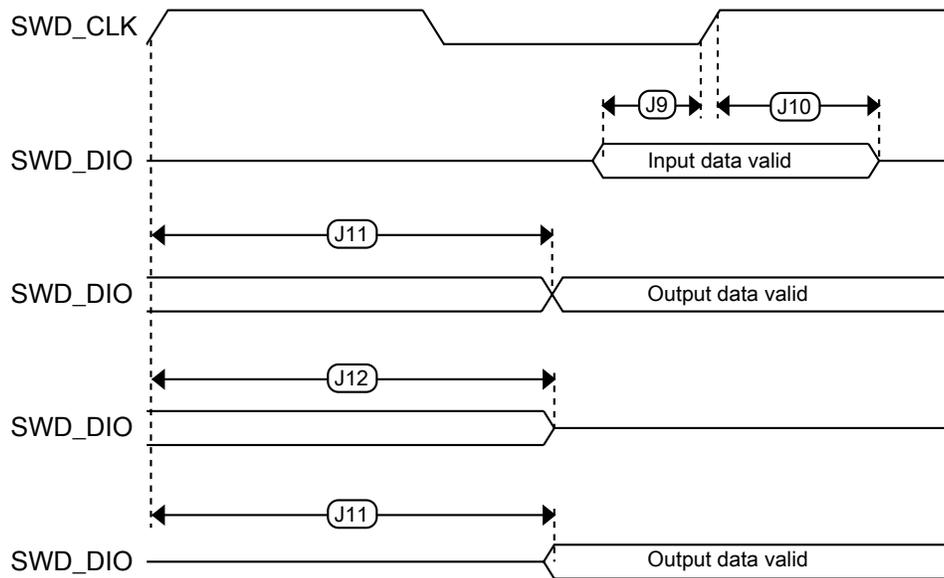
Figure 8. Serial wire data timing
