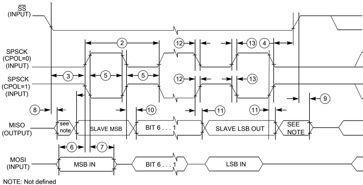
**Figure 15. SPI slave mode timing (CPHA = 0)**
