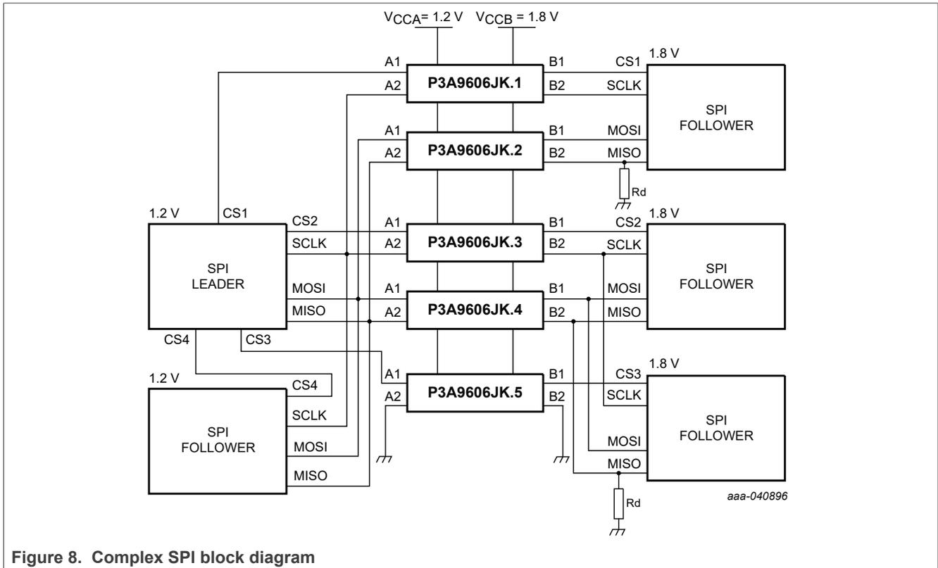
Figure 8. Complex SPI block diagram
