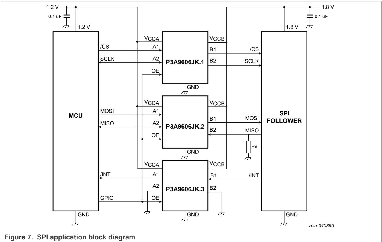
Figure 7. SPI application block diagram
