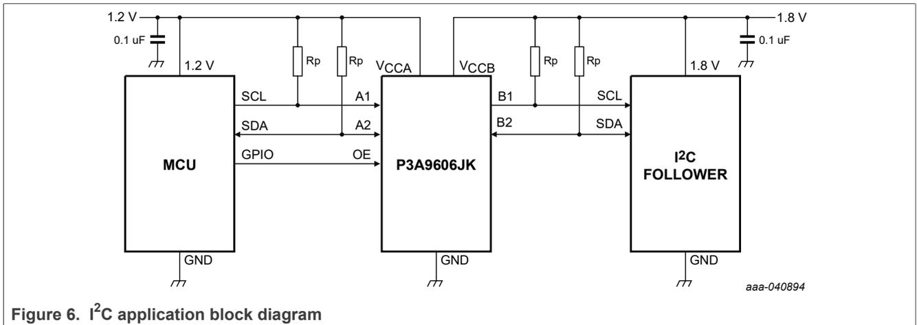
Figure 6. I<sup>2</sup>C application block diagram
