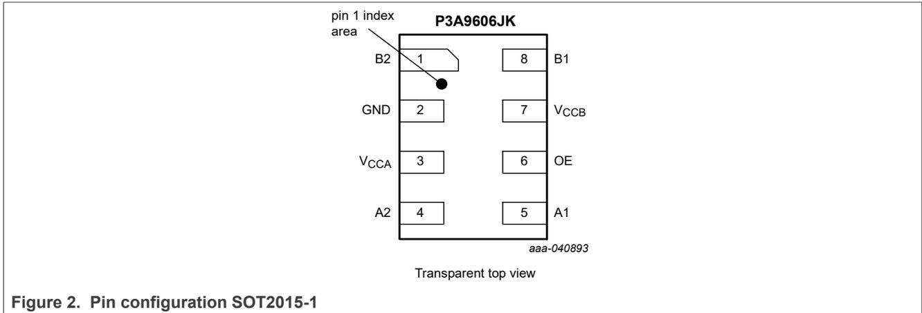
Figure 2. Pin configuration SOT2015-1
