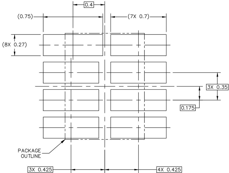
PCB DESIGN GUIDELINES – SOLDER MASK OPENING PATTERN
