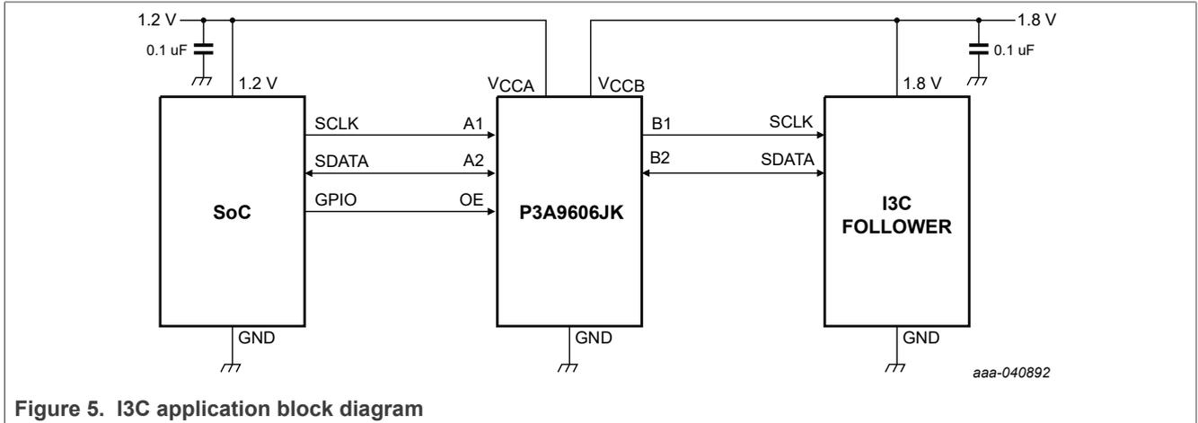
Figure 5. I3C application block diagram
